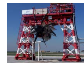
Open air test bench for A400M acoustic testing
