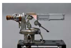
Mars Science Laboratory High Gain Antenna Gimbal - HGAG
