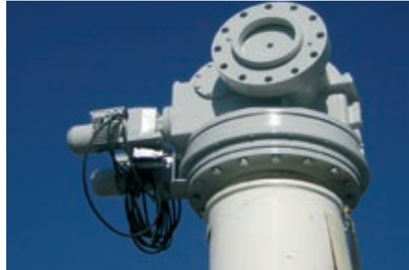
SENER's heliostat axis drive mechanism.
